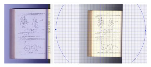
Figure 4. Splitting of pages (left) and automatic de-skewing of one page (right)
